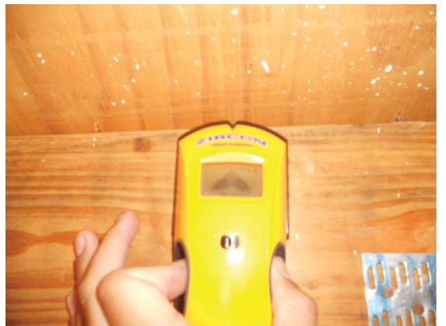
Roof Deck Attachment:- Nail Detection
